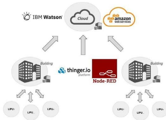
Fig. 1 - Architecture with platform integration.
