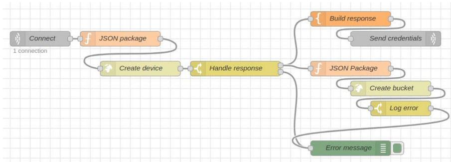
Fig. 2 - Node registration implementation in Node-RED.
