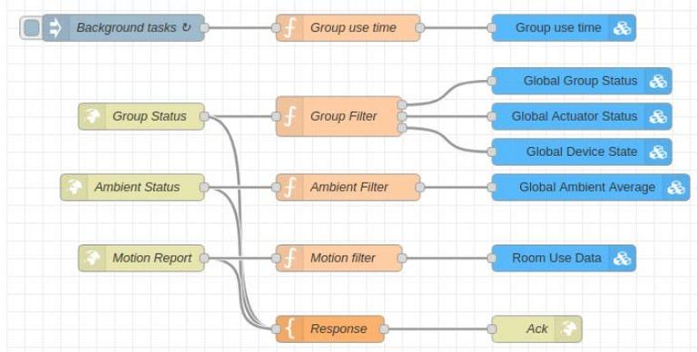
Fig. 3 - Data processing implementation in Node-RED.
