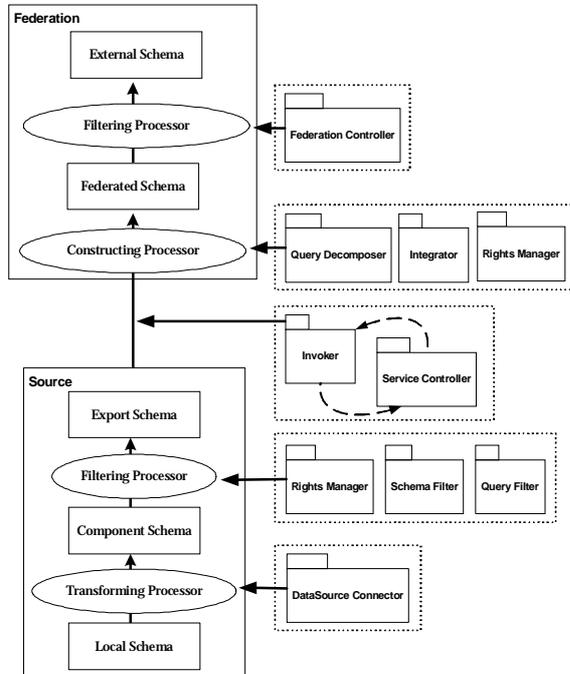
Figure 8: Designed Architecture - Five-level Architecture Mapping
