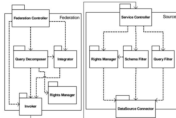
**Figure 7: Designed Architecture**
