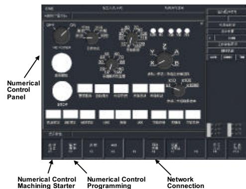
Fig.4 Web-based Remote Numerical Control Monitor
