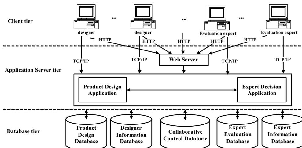
Fig.1. Three-tier Architecture in CPD System
