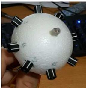
Figure 3: The semi-sphere shape sensor showing the position of the LDRs.
